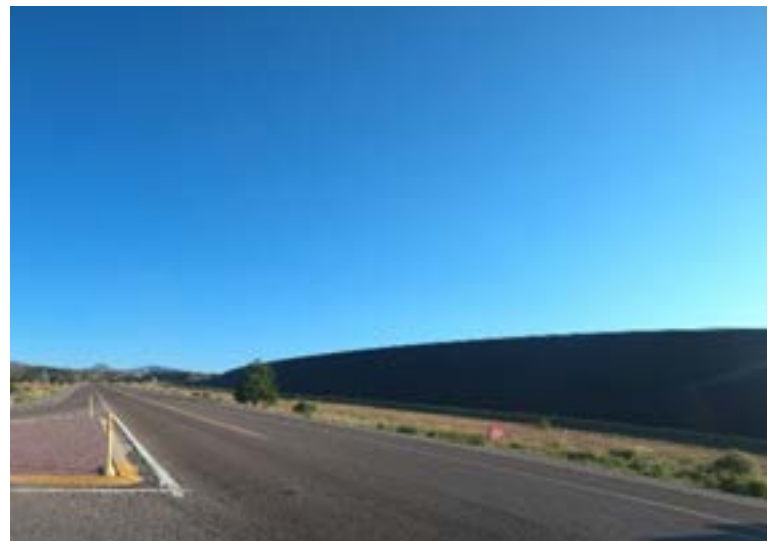
Looking north along NM 22 from the stop bar at Intersection 12.2. Drivers are challenged to see vehicles approaching from the distance, especially at high speeds and in the morning hours. (Photo credit: Merrill J. Yazzie, Pueblo de Cochiti)
